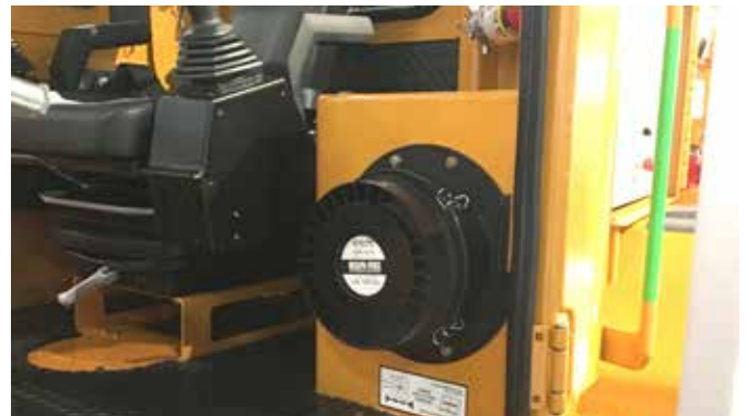
Figure 4- RESPA® FFX2 Recirculation Filtration unit- replaces HVAC Panel Filter
