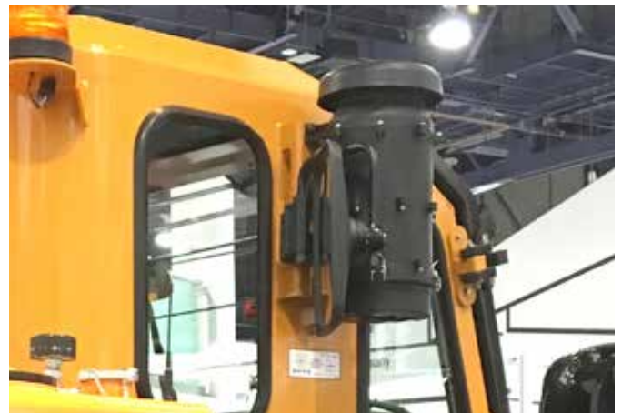
Figure 3- Cabin fitted with RESPA® CF2 External Air Unit
