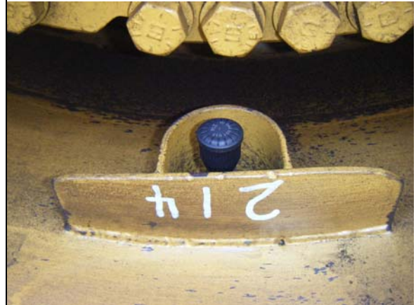
Figure 4 Correct Mounting of Large Bore Sensors on HME. Solid Air Valve Stem with Protection.
