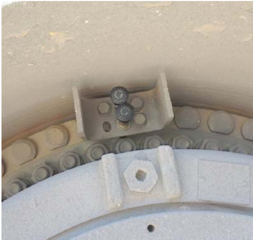
Figure 3 Correct Mounting of Large Bore Sensors on HME. Solid Air Valve Stem with Protection.
