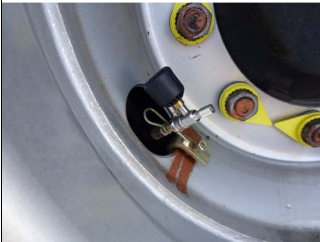
Figure 5 Correct Mounting of Small Bore Sensors on Truck / Trailer Tyre (note "T" Valve).
