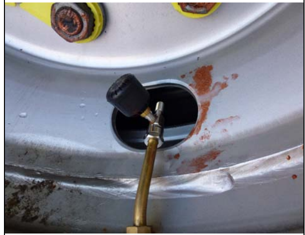
Figure 6 Correct Mounting of Small Bore Sensors on Truck / Trailer Tyre (note "T" Valve).
