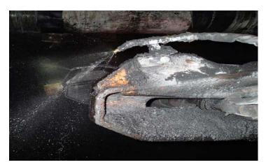
Figure 29: Single spray located on the tail of the Continuous miner.
