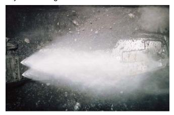
Figure 22: Side sprays on Tailgate ranging arm
