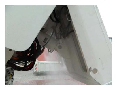
Figure 10: Rear caving door sprays
