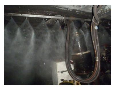
Figure 9: Face partition sprays installed on a shield canopy
