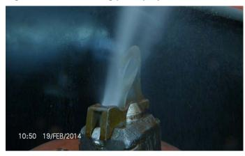
Figure 15: Back flushing pick spray
