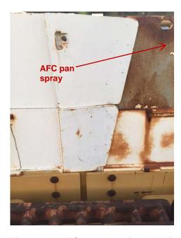
Figure 11: AFC pan spray installed in spill tray
