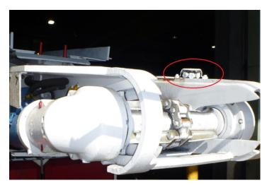
Figure 30: Spray bank located on the tail of the Continuous miner.
