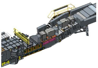
Figure 3: BSL fitted with two scrubber fan units
