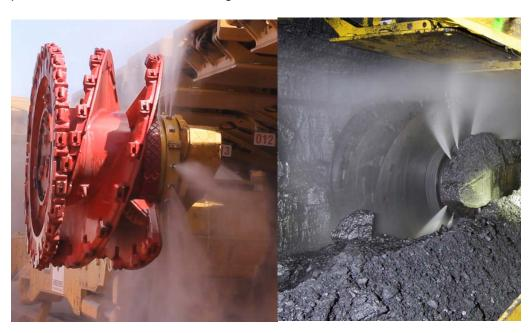
Figure 17: Ranging arm sprays
