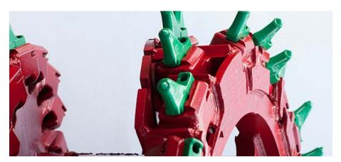
Figure 19: Shearer drum fitted with Radial picks
