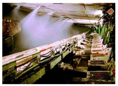
Figure 6: Shield canopy sprays
