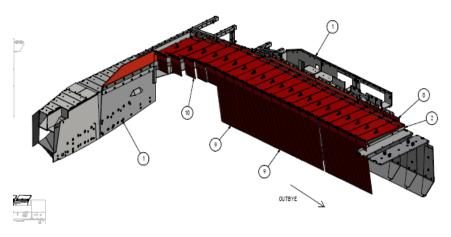
Figure 13: BSL/AFC transfer containment covers - view from block side
