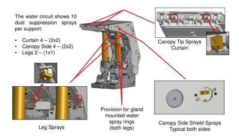
Figure 7: Dust suppression spray positions
