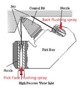
Figure 16: Pick and flushing spray position
