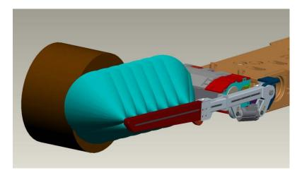
Figure 20: Shearer clearer spray pattern
