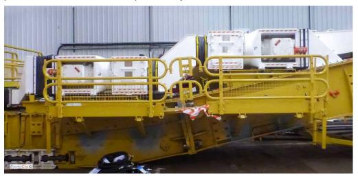
Figure 2: Scrubber fan system mounted on BSL
