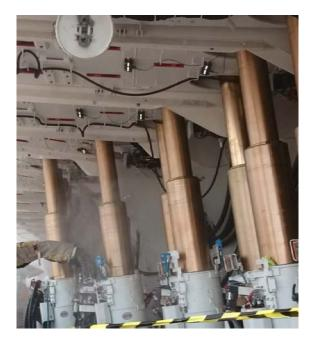
Figure 8: Leg sprays activating during LAS cycle
