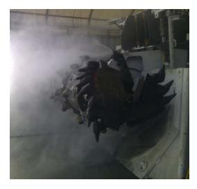
Figure 28: Cutter head sprays
