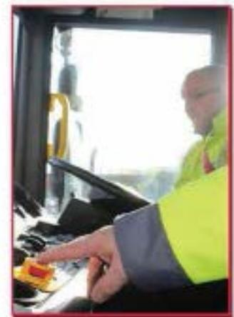
The **VT StopSafe**, effectively reduces the vehicle's speed while simultaneously bringing it to a controlled stop using the braking system. The system is activated using a secure emergency button installed to the vehicle dashboard, allowing the crew (or passenger) to react to an emergency situation.
