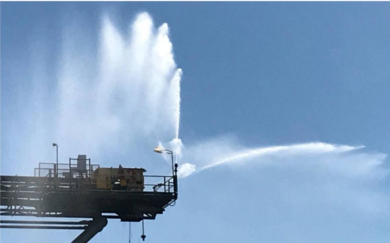
**Figure 4. Cannons on conveyor delivery points to suppress stockpile dust**
