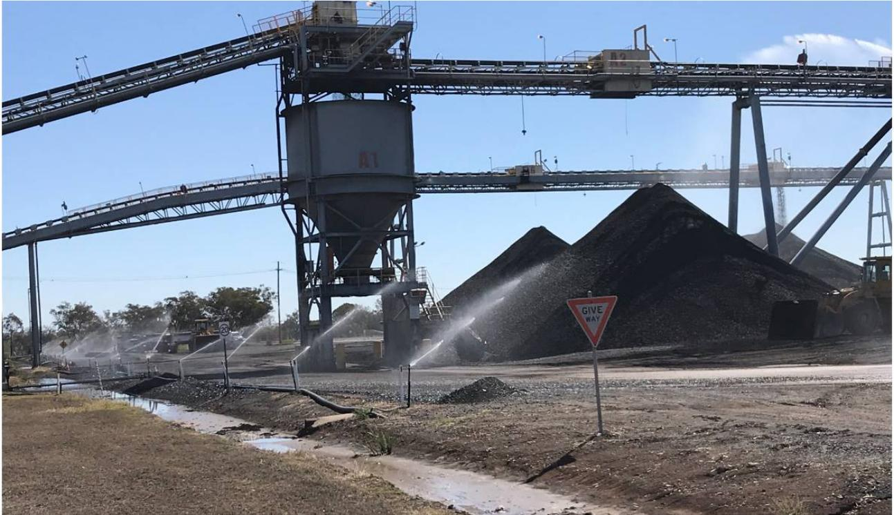
**Figure 12. Sprinklers suppressing dust on roadways**
