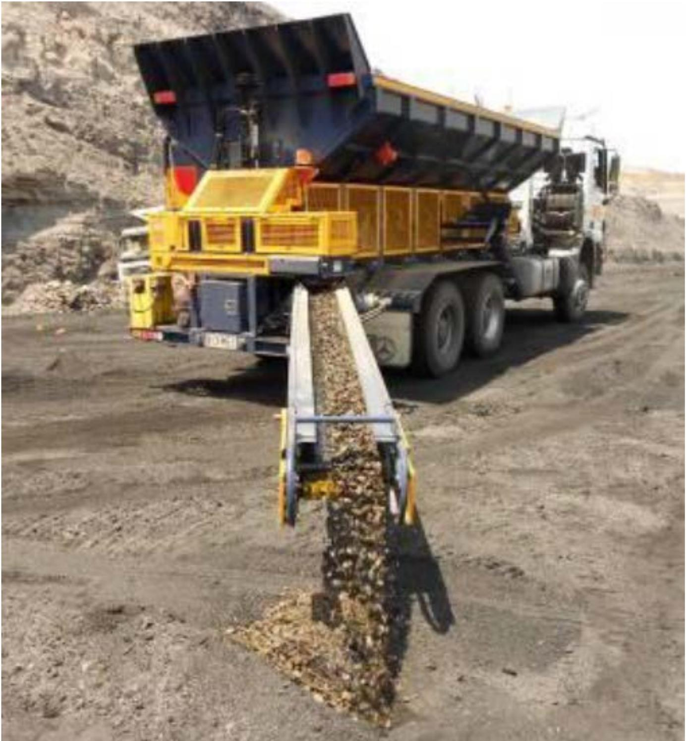
Figure 15. Stemming truck delivering stemming to blast hole
