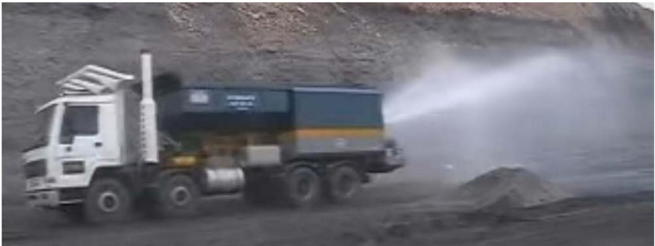
**Figure 13. Watering shot bench down to suppress surface dust**
