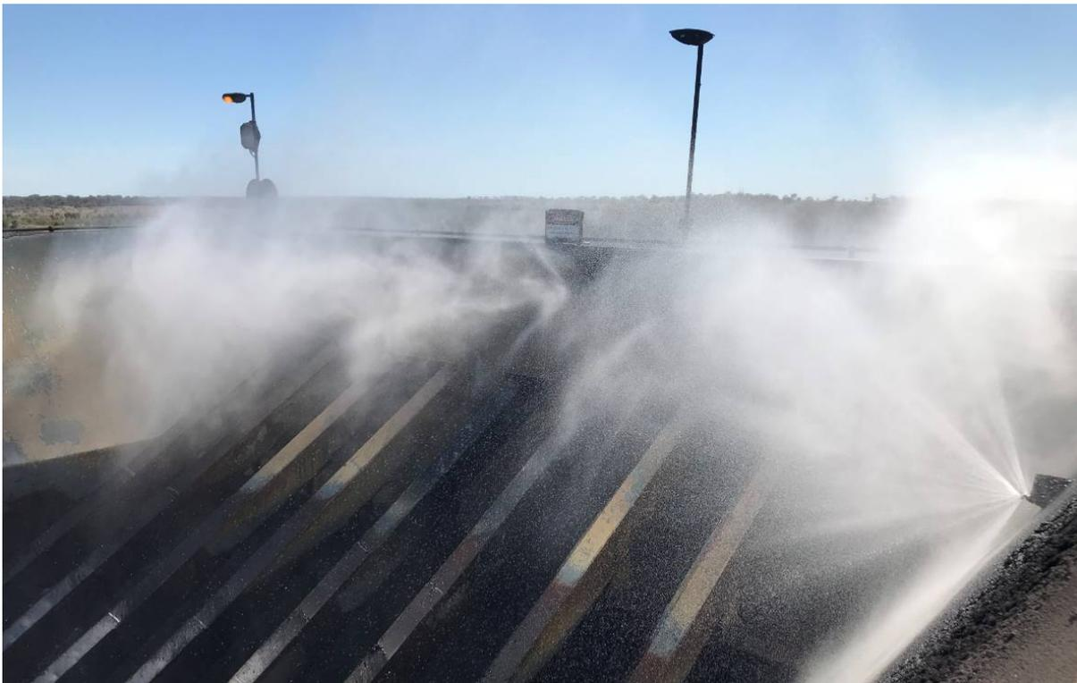
**Figure 2. Sprays on dump stations**
