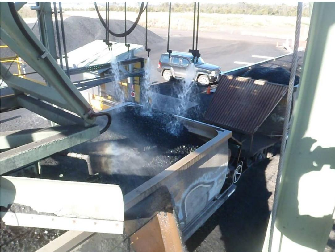
**Figure 17. Profiler and Veneering Solution being applied**
