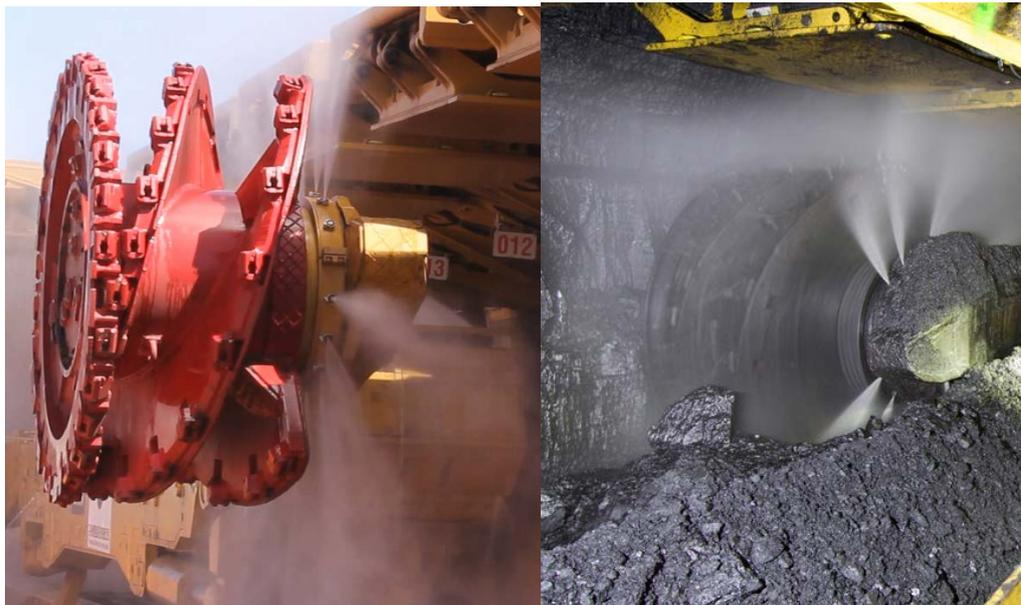
**Figure 17: Ranging arm sprays**
