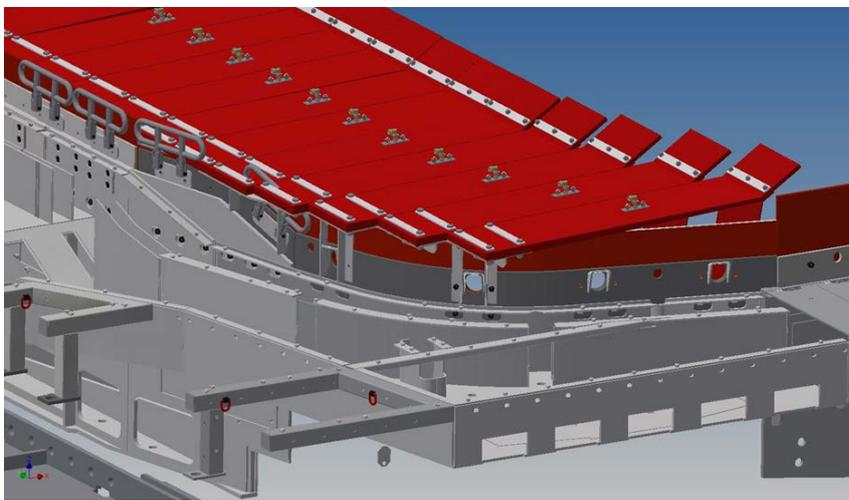
Figure 12: BSL/AFC transfer containment covers – view from goaf side
