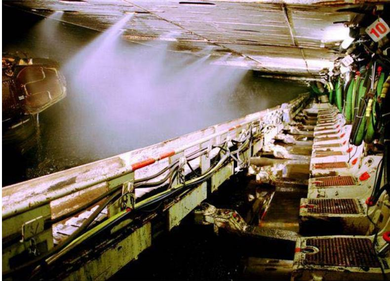
Figure 6: Shield canopy sprays
