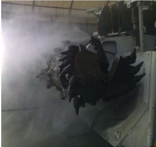
Figure 28: Cutter head sprays
