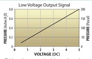
This low voltage output signal chart can be used to calibrate real-time pressure data when sent to a computer or telemetric system. A more detailed version of the chart is available on www.sy-klone.com.
