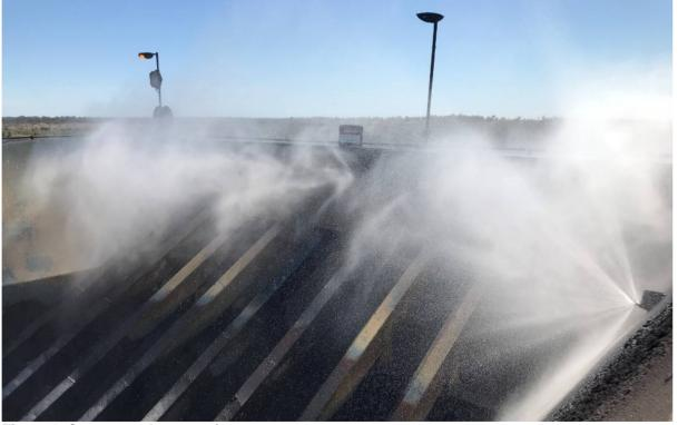
Figure 2. Sprays on dump stations
