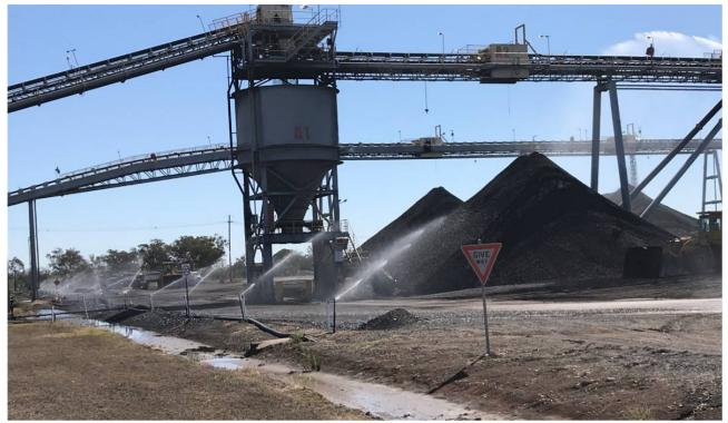
Figure 12. Sprinklers suppressing dust on roadways
