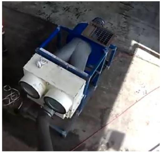
Figure 9. Portable extraction unit
