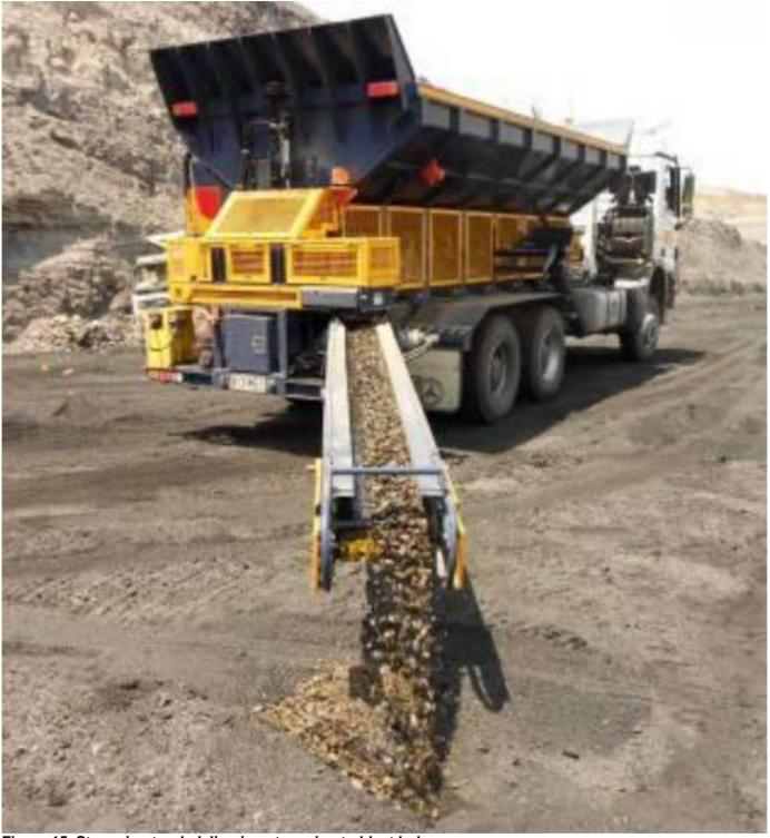
Figure 15. Stemming truck delivering stemming to blast hole
