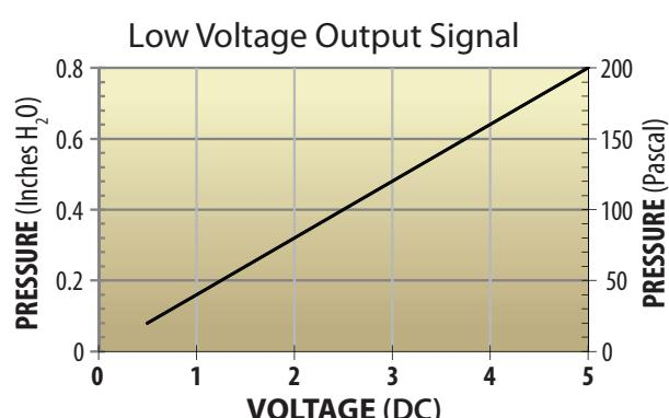
This low voltage output signal chart can be used to calibrate real-time pressure data when sent to a computer or telemetric system. A more detailed version of the chart is available on [www.sy-klone.com](http://www.sy-klone.com).
