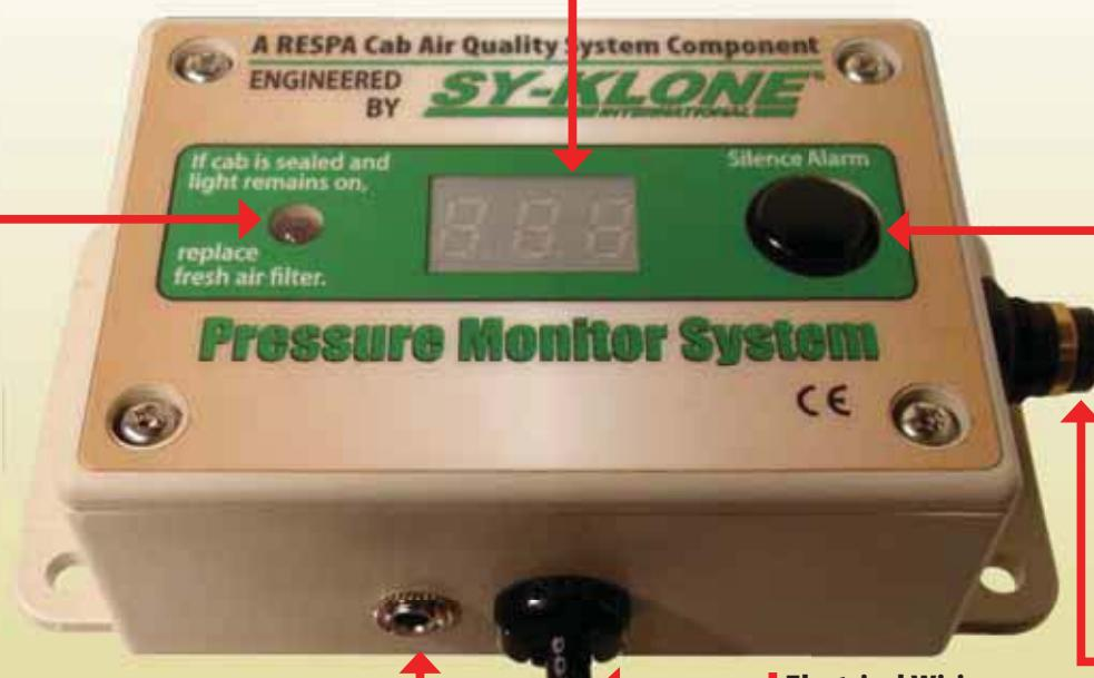
**Low Voltage Pressure Signal Port:** The unit includes a 0 to 5 volt output signal that can stream realtime pressure information to an on-board computer. The 1/8" mono plug signal port puts out a low power voltage signal that varies with the pressure reading (see technical specifications for details).
