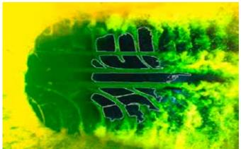
Figure 2: Tyre Contact Pattern- 100% Pressure Set- point
