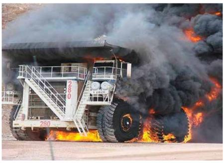
Figure 1: DTruck Tyre Fire- major Asset loss
