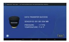
The **Read Individual Sensor** feature allows the technician to hold the tablet at a reasonable distance from the tyre sensor and tap on the on-screen sensor image to trigger the data transfer.
