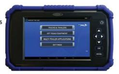
One-Click<sup>™</sup> Transceiver to quickly access and record digital tyre pressure and temperature data from Individual Sensor Readings, Equipment Walk Arounds or by transferring the data from the SmartLink<sup>™</sup> One-Click<sup>™</sup> Transceiver.
