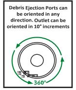
Debris Ejection Ports
