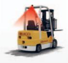
In confined areas or unclear situations it is often difficult to estimate the space behind the forklift truck accurately. Also, frequent driving in reverse causes strain on the driver's neck- and shoulder muscles. The **Rearview** system ensures a safe environment in which the physical strain for the driver is minimal.
