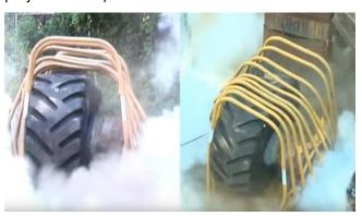
The tyres above are undergoing a controlled test and have exploded and destroyed the steel safety cage around them. Note that these tyres are half the size of a crane tyre. The tyre below is only a truck tyre, but it's clear that the test dummy won't be used again.
