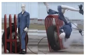
The electrical arcing events described in Bulletin 207 have been known to cause tyre pyrolysis. Throw lightning strike into the mix also. Although it's rare, it still happens.
