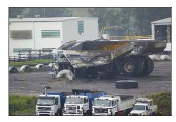
These dump trucks weigh 130t unloaded, and have a loaded weight of 320t, so they are somewhat bigger than any of the cranes that travel on our roads. They carry a larger tyre sizes as well. Yet the potential for a similar event is possible. When the size of one of the tyre sections that blew off is shown up close below, it's easy to appreciate that that a greater understanding of this phenomenon is something that all of us in the crane and related industries should be aware of.
