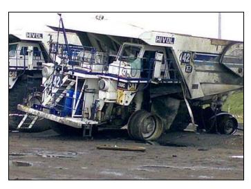
The machine pictured above is a Cat 789C and the tyres were said to have blown off the truck minutes after the lightning strike. One wheel assembly weighing 1.6t was thrown about 100m from the machine, and other components found up to 275m away as seen in the image below. The truck also suffered extensive damage including major driveline damage and the door & glass blown open.
