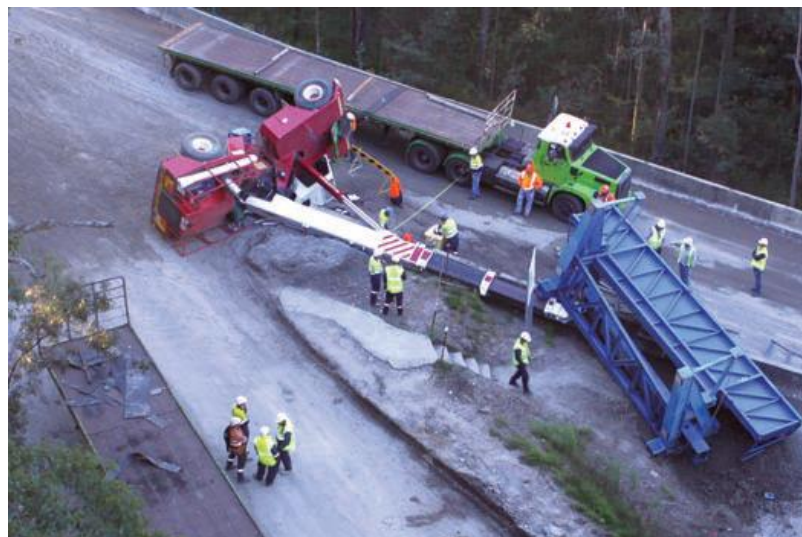
Figure 1: Articulated Crane Rollover when Carrying a Load [1]
