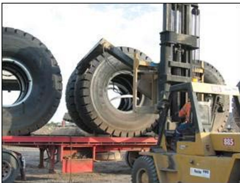
Image 4: Unloading tyre using fit-for-purpose equipment
