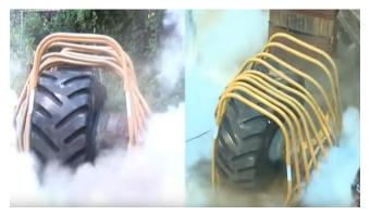
The tyres above are undergoing a controlled test and have exploded and destroyed the steel safety cage around them. Note that these tyres are half the size of a crane tyre. The tyre below is only a truck tyre, but it's clear that the test dummy won't be used again.
