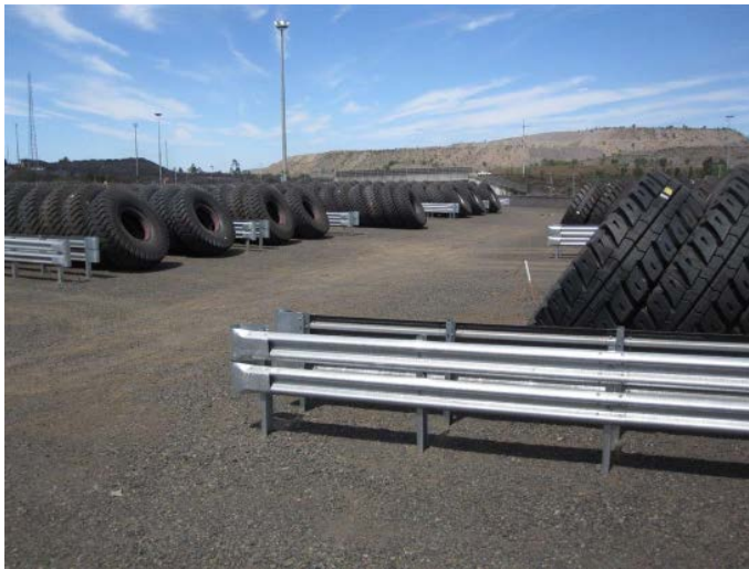
Image 5: Vertical tyre storage showing inspection corridors and segregation
