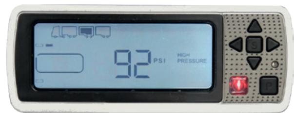
HIGH PRESSURE ALARM
