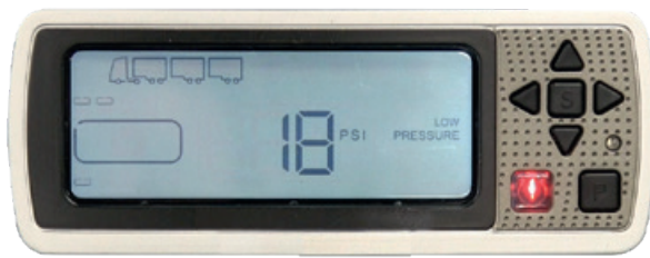
LOW PRESSURE ALARM
