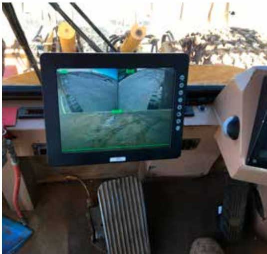
Figure 5: Operator Visibility- Rear / LHSide / RHSide views with Radar Detection warning overlays.
