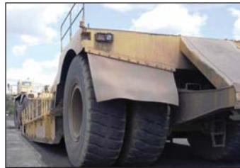
A utility cab was recently crushed beneath a projecting 'tow hitch' at the rear of a low-loader.
