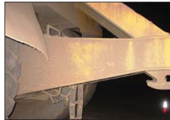
A utility cab was recently crushed beneath a projecting 'tow hitch' at the rear of a low-loader.
